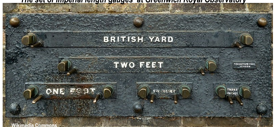
The set of imperial length gauges at Greenwich Royal Observatory
